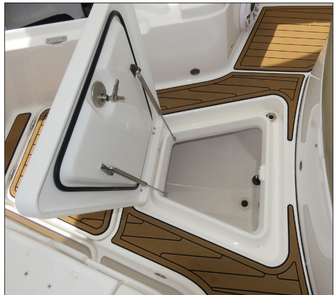
Forward Fishbox Drain & Drain Rails
