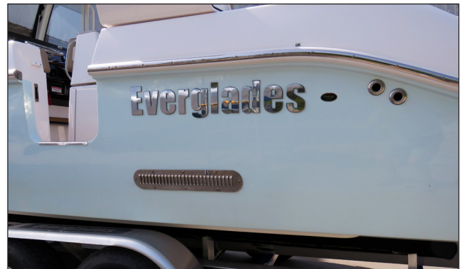
Hull Side Scupper Drain Thru-hull Grate
