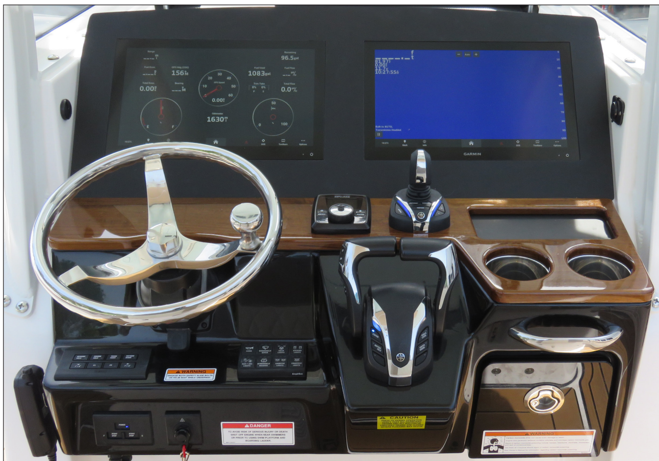
Helm Switch Panels
