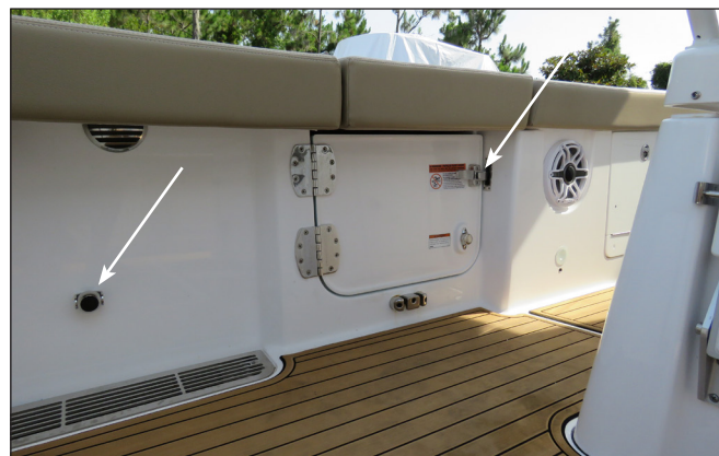
Side Boarding Door and Gate Closed Magnetic Latch & Door Latch w/ Safety Pin
