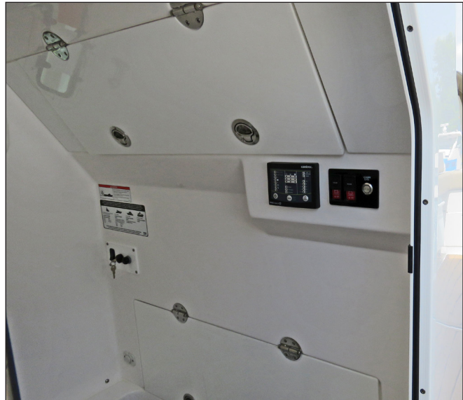
Helm Equipment Access Doors in Head Compartment
