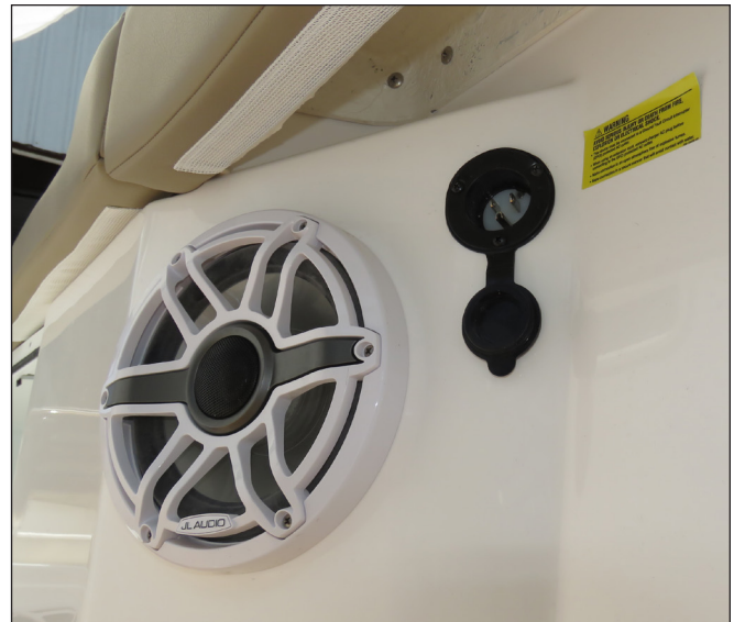
Shore Power Cable Inlet Connection
