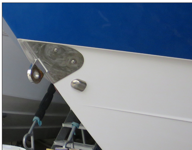
Rope Locker Drain Fitting in Hull Side
