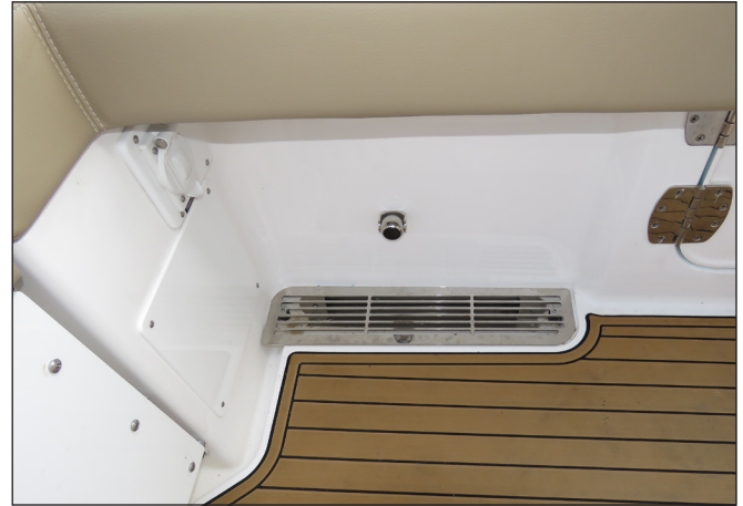
Typical Scupper Drains & Drain Rail
