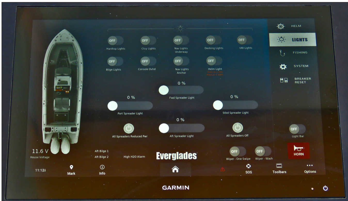
Typical Digital Switch Control Screen
