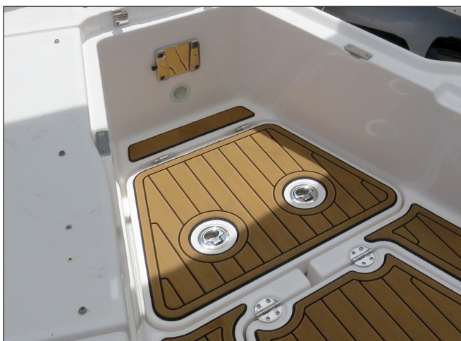
Bow Filler Table Secured to Cockpit Sole
