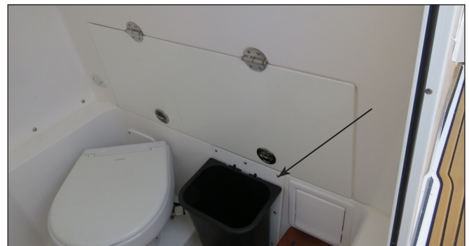
Removable Panel Provides Access to Bilge Below Helm
