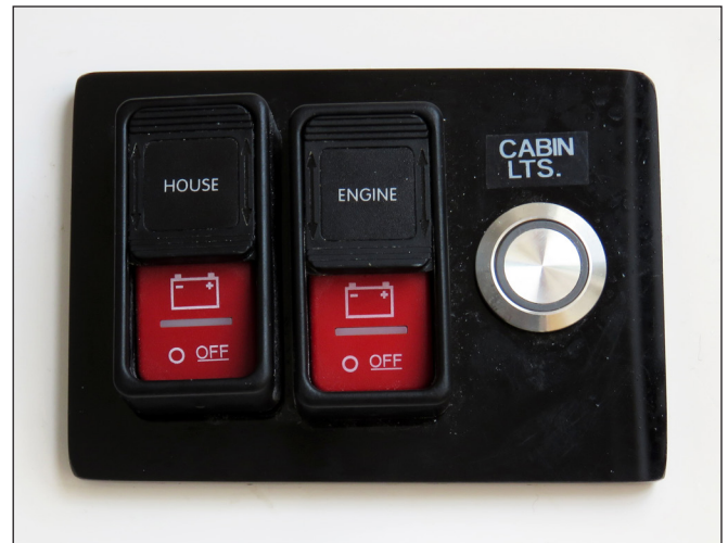
Battery Switches on Panel in the Head Compartment
