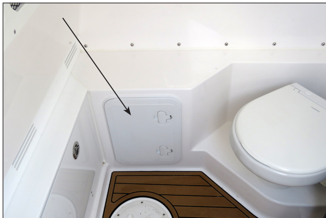
Removable access Hatch on Starboard Side
