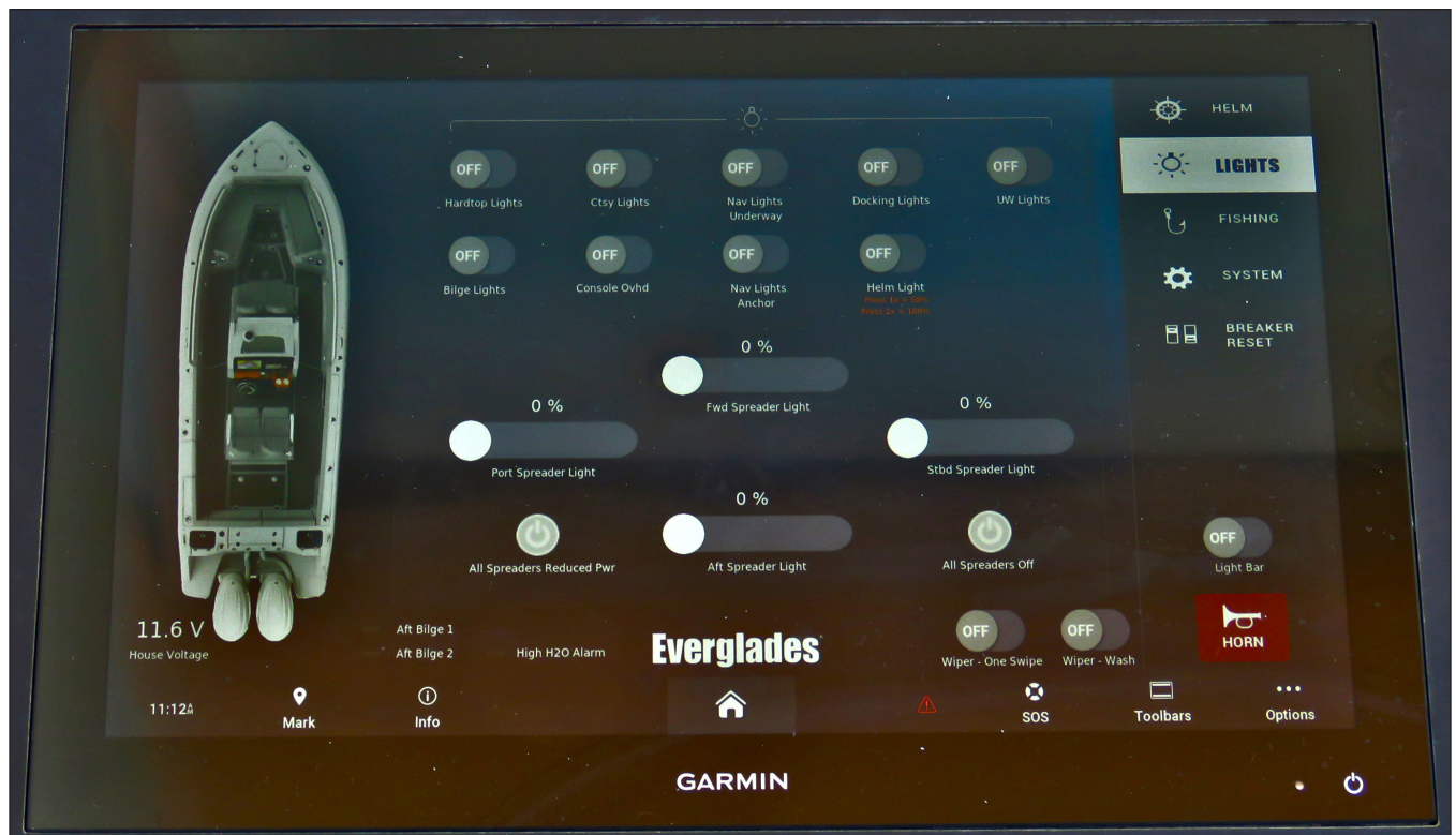
Typical Switches in Helm Touch Screen Display
