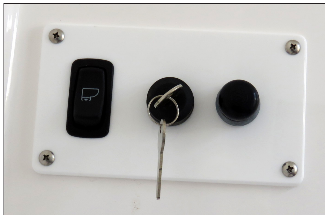
Toilet Fill/Flush Switch, Key Activated Lockout Switch & Macerator Discharge Pump Switch
