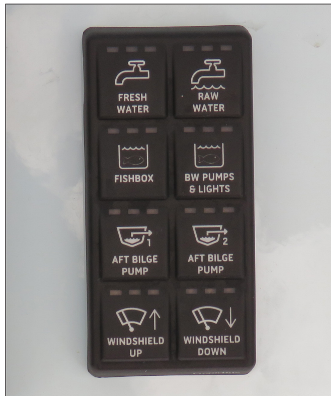
Starboard Hardtop Switch Panel
