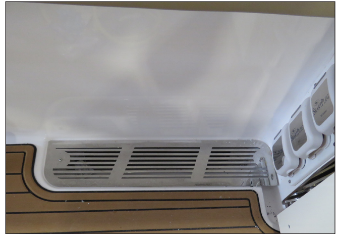
Typical Scupper Drains & Drain Rail
