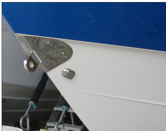
Rope Locker Drain Fitting in Hull Side
