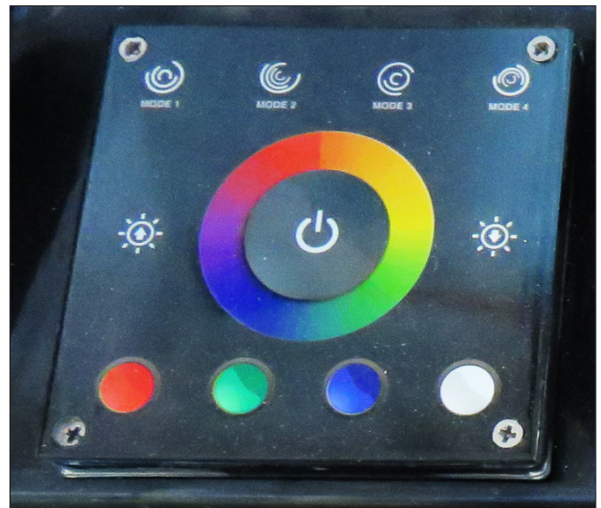
Light Mode Control Panel
