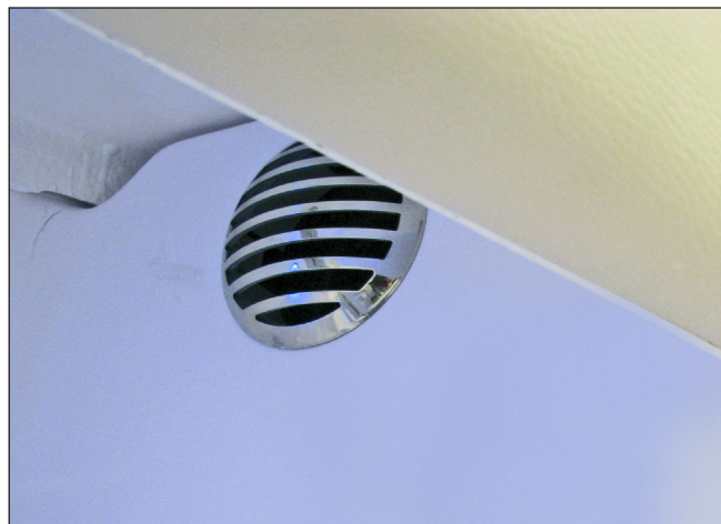
Typical Free Air Vent Below Gunnels in Cockpit
