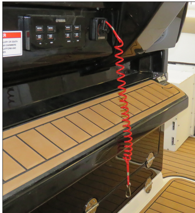
Triple Engine Stop Switch Lanyard
