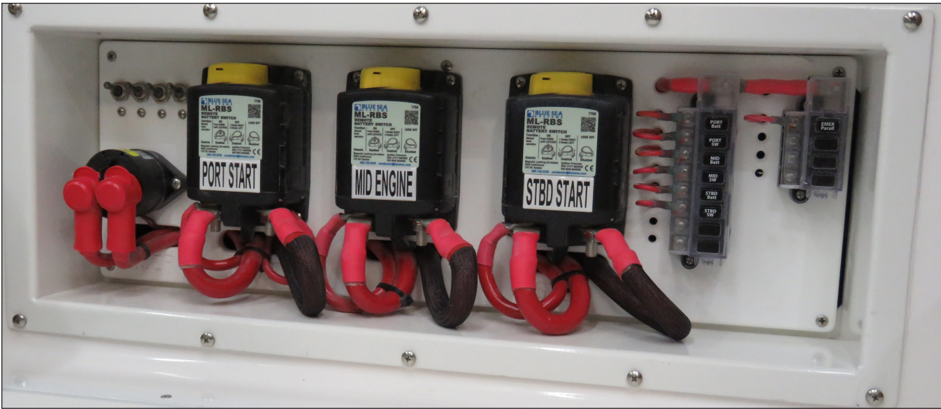
Engine Battery switches & Battery Parallel Switch, Fuse Panels for Remote Battery & Parallel Switches Located Behind the Starboard Cabin V-Berth Backrest Cushion
