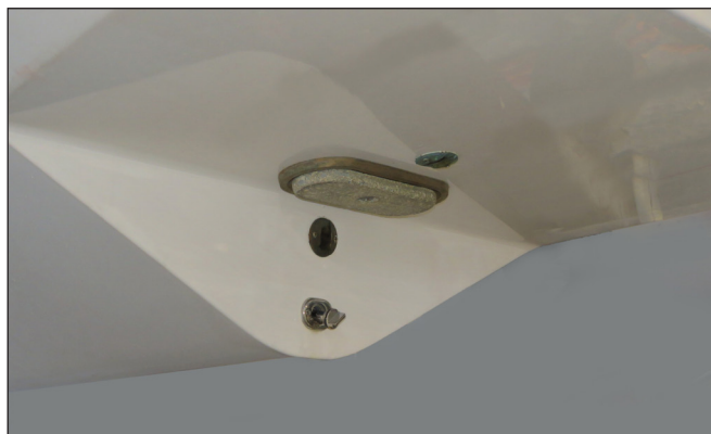
Typical Transom Anode
