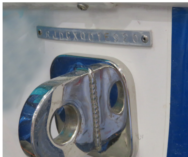
Hull ID # On Starboard Side of Transom
