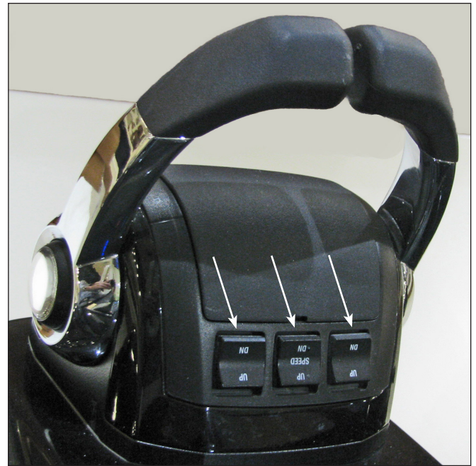
Yamaha Helm Master Control Engine Trim Switches
