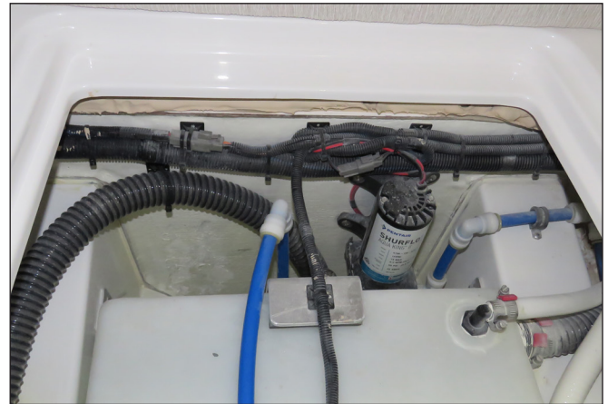
Fresh Water Pump & Tank
