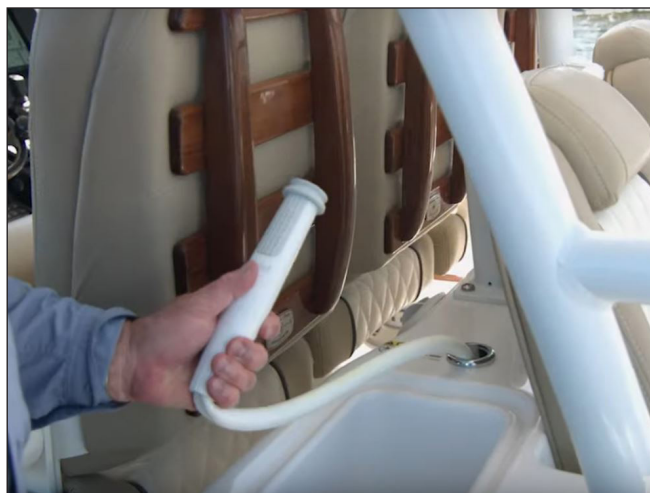
Cockpit Fresh Water Shower in Mezzanine
