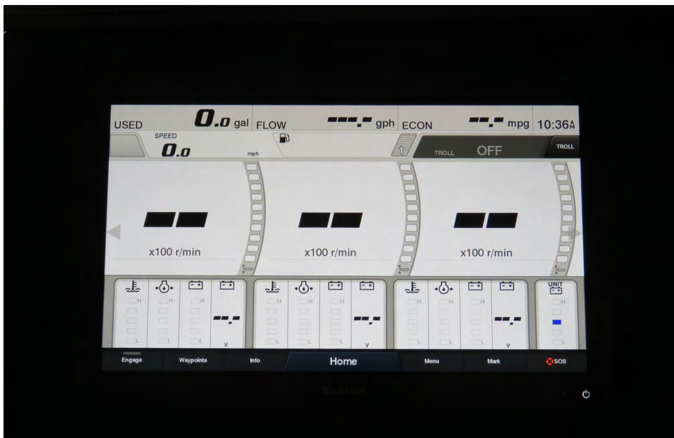
Typical Digital Engine Monitoring Screen On a Garmin Display
