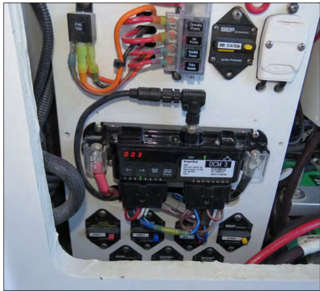
Digital Switch Control Module & Main Circuit Breakers
