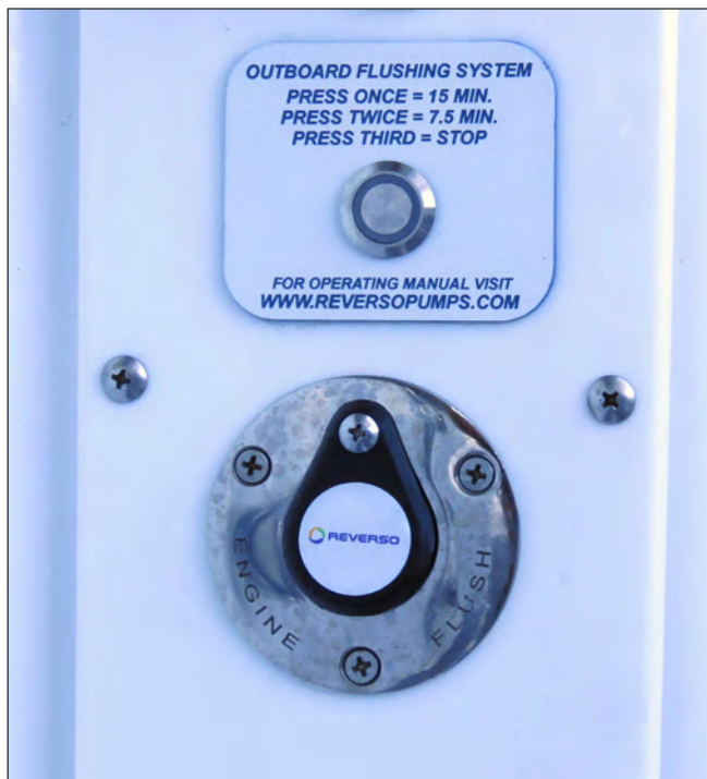
Typical Engine Flushing System & Shore Water Connection
