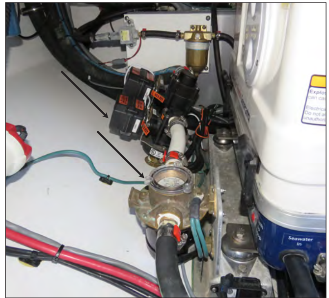
Typical Generator Raw Water Electrically Activated Thru-Hull Valve & Strainer
