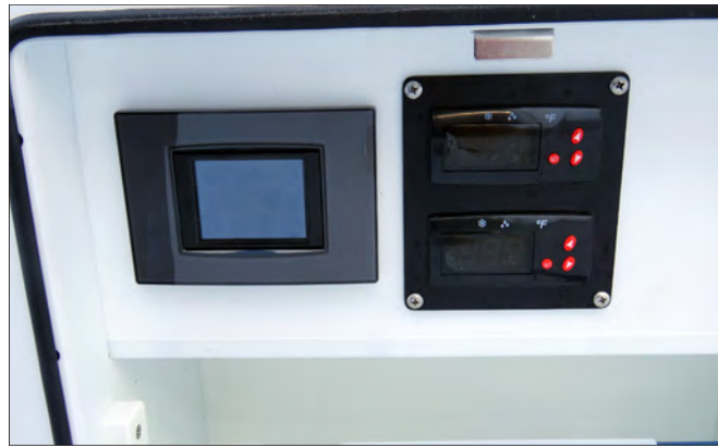
Cockpit Air Conditioner & Freezer Plate Control Panels
