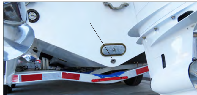
Transom Garboard Drain Plug
