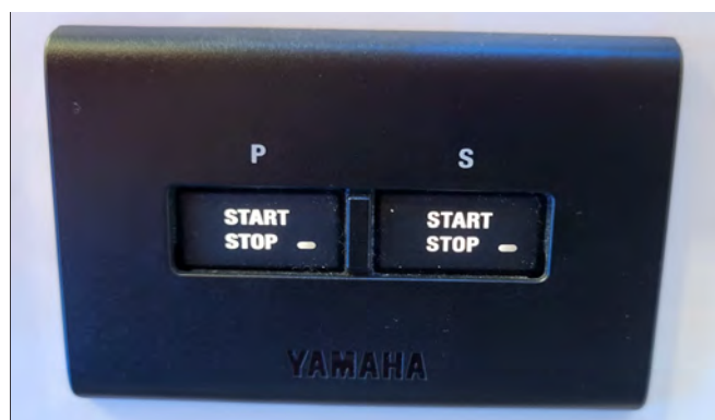
Typical Yamaha Helm Master Twin Engine START/STOP Switch Panel
