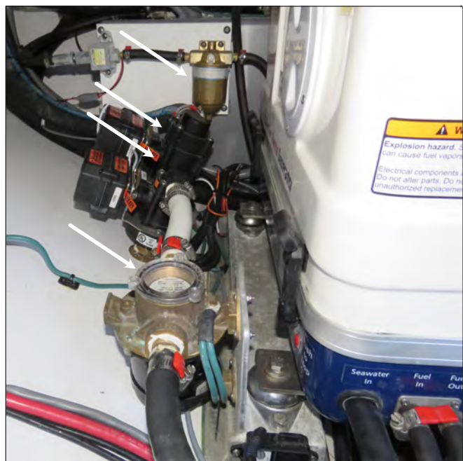
Generator Sea Strainer, Fuel Filter & Electrically Activated Thru-Hull Valves
