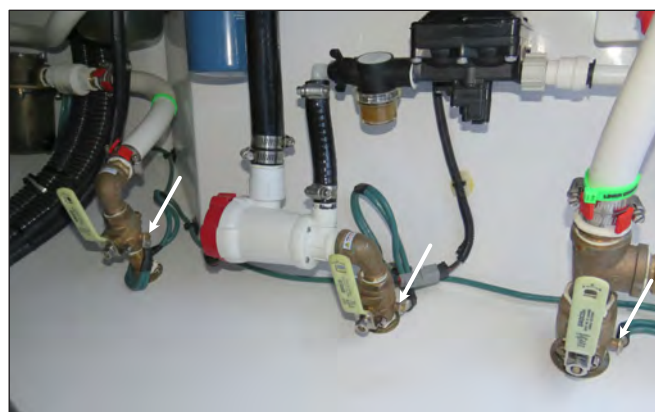
Typical Bonding Wires & Connections
