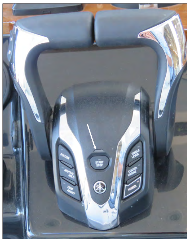
Yamaha Control All Engine Start/Stop Button
