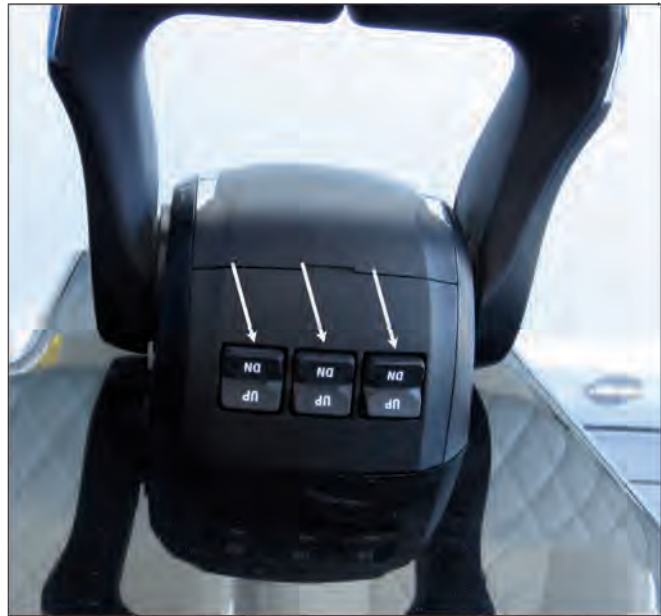
Typical Yamaha Control Triple Engine Trim Switches
