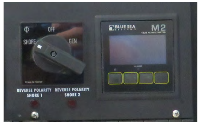
SHORE/OFF/GENERATOR Switch & Multimeter
