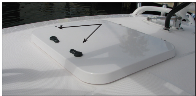
Upper Station Access Hatch Note exterior access hatch cam latch levers.
