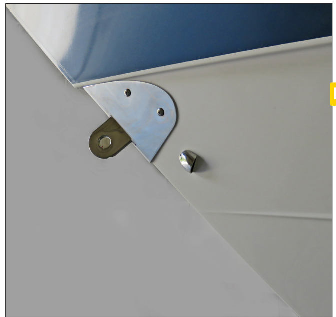
Rope Locker Drain Fitting in Hull Side
