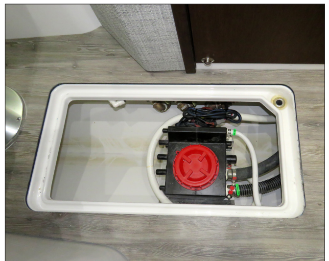
Removable Cabin Floor Panel & Cabin Drain Sump System
