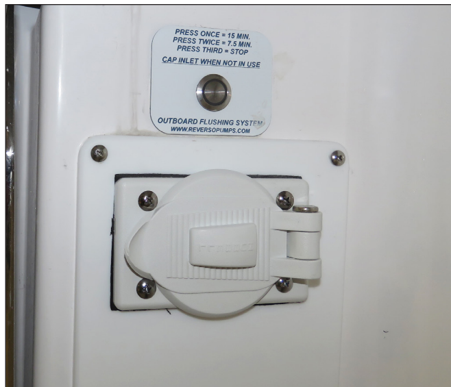
Typical Outboard Flushing System Control Button
