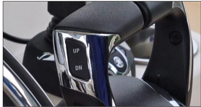
Tilt Trim Switch on Control Lever
