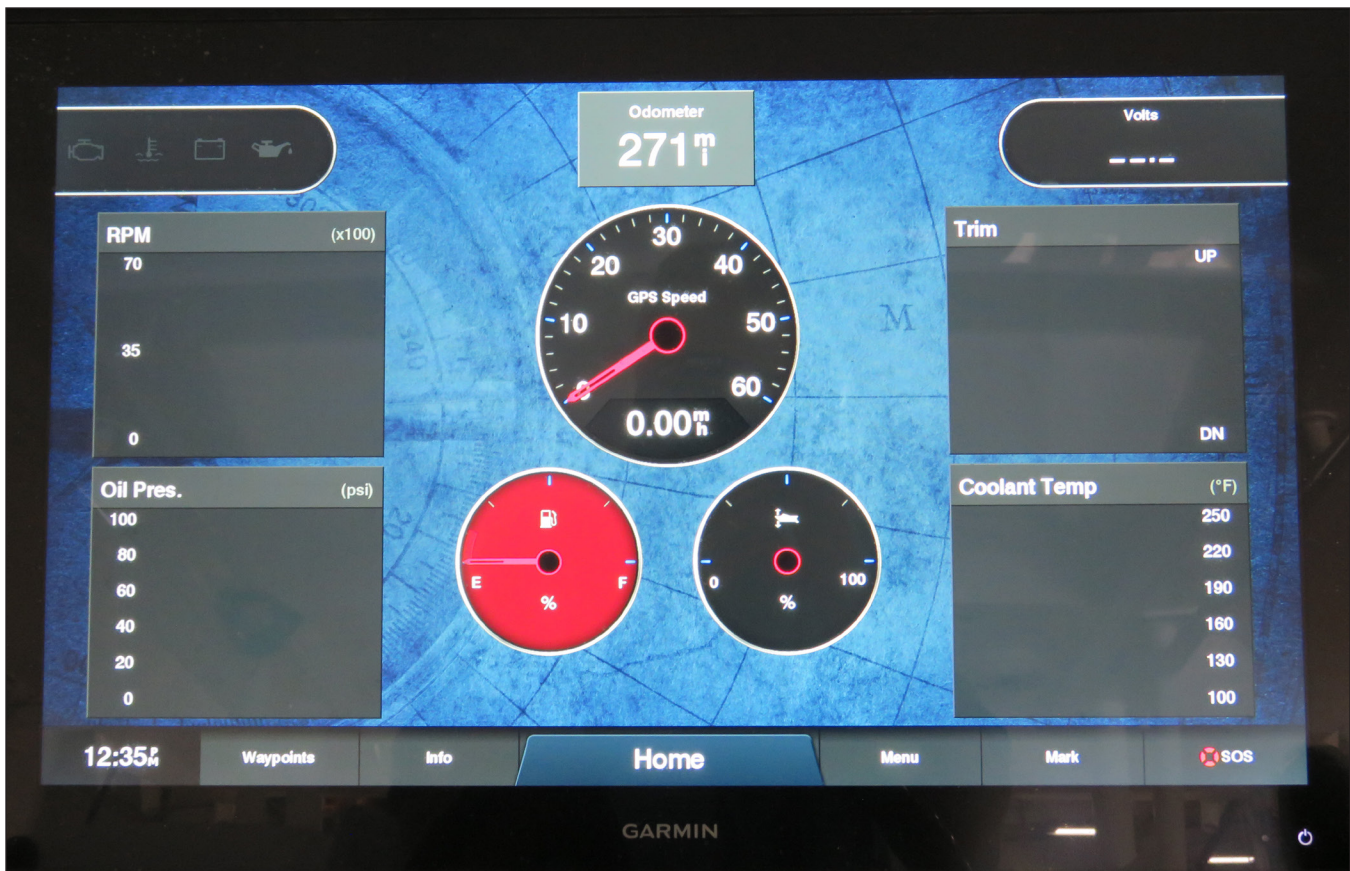
Typical Analog & Graphical Engine Monitoring Screen On a Garmin Display
