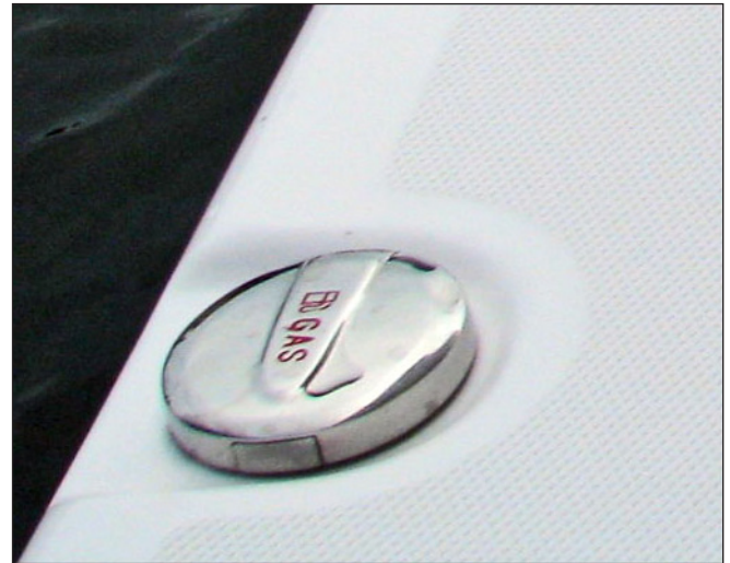
Typical Fuel Fill
