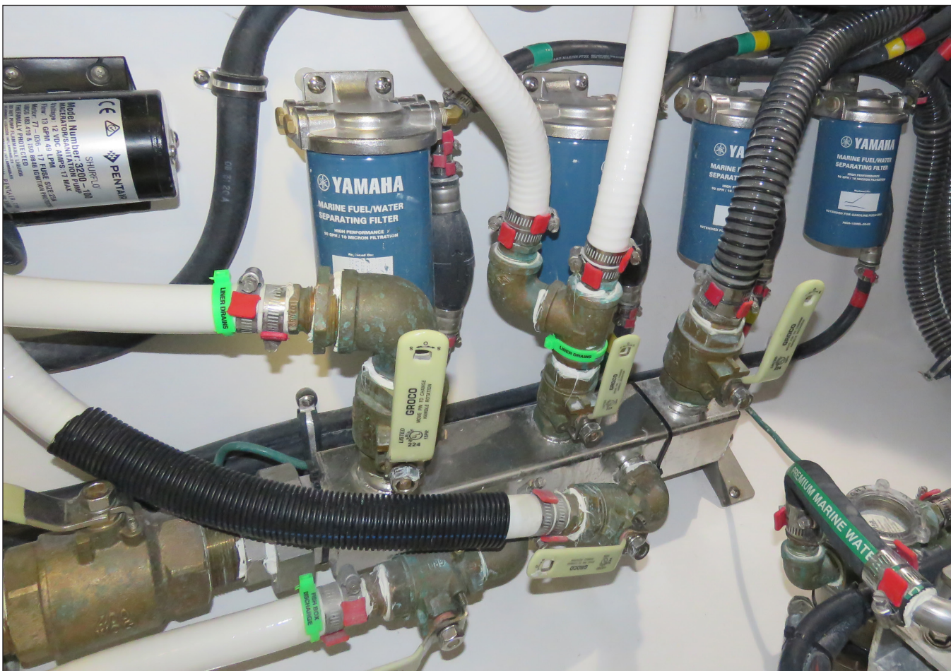
Typical Yamaha Engine Fuel Filters & Primer Bulbs
