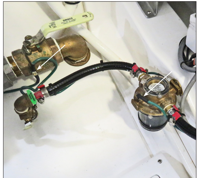
Typical Bonding Wires & Connections
