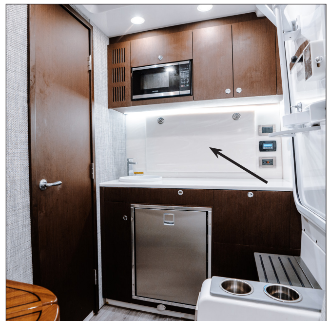
Helm Equipment Access Hatch in Aft Cabin Bulkhead
