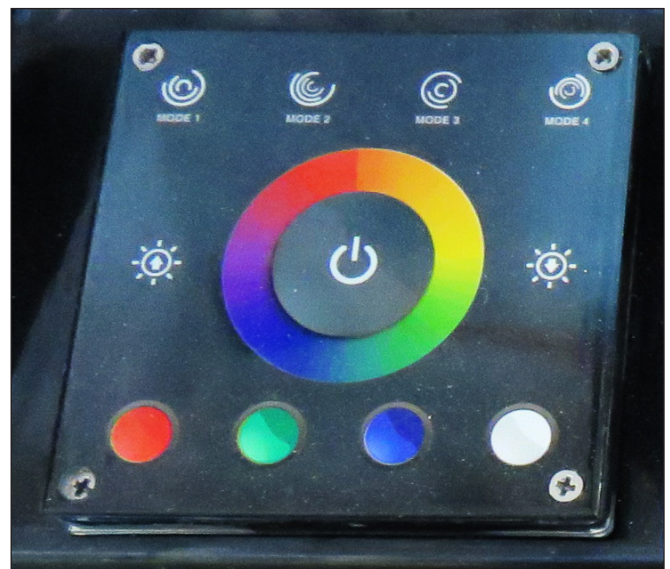
Light Mode Control Panel
