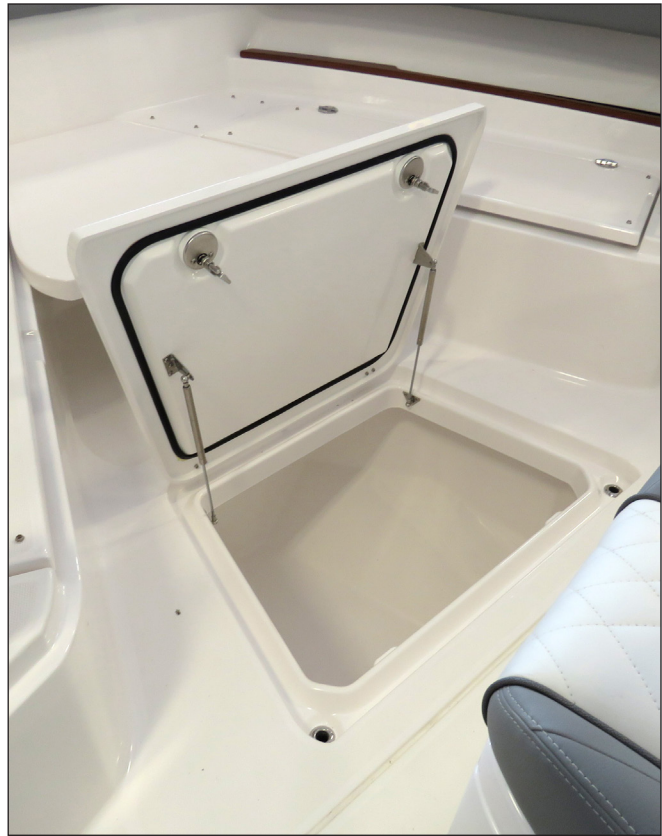
Forward Fishbox Hatch & Drain Rails
