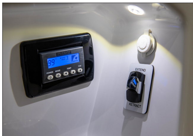
Typical Cockpit Air Conditioner Control Panel
