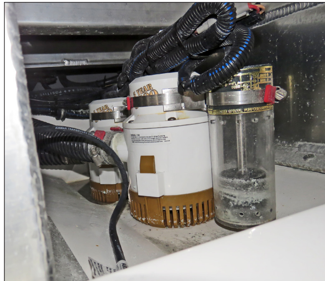
Aft Bilge Pumps & Automatic Switches
