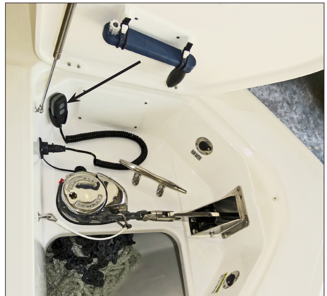
Windlass Control Switch
