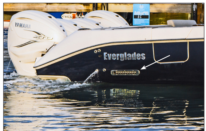
Hull Side Scupper Drain Thru-hull Grate
