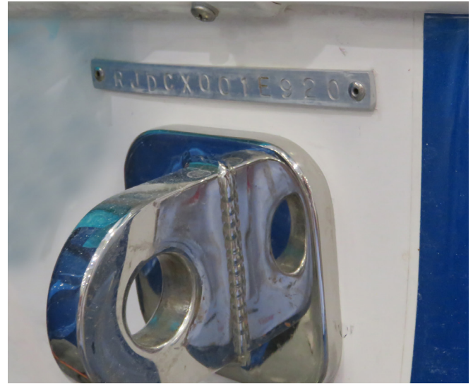
Typical Hull ID # On Starboard Side of Transom
