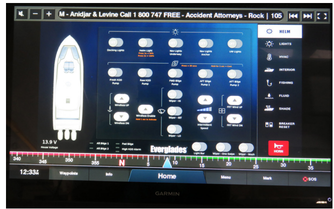
Typical Switches in the Helm Switch Touchscreen Display
