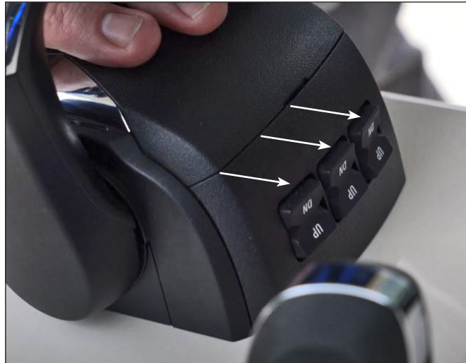
Yamaha Helm Master Control Engine Trim Switches
