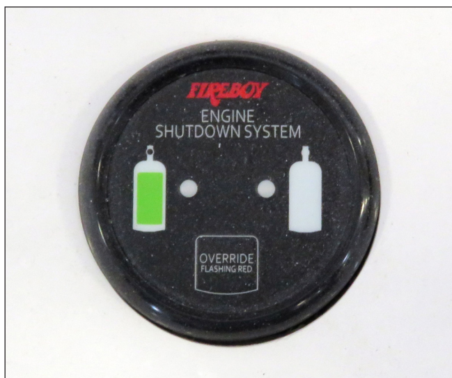
Fire Extinguisher Panel In Helm
