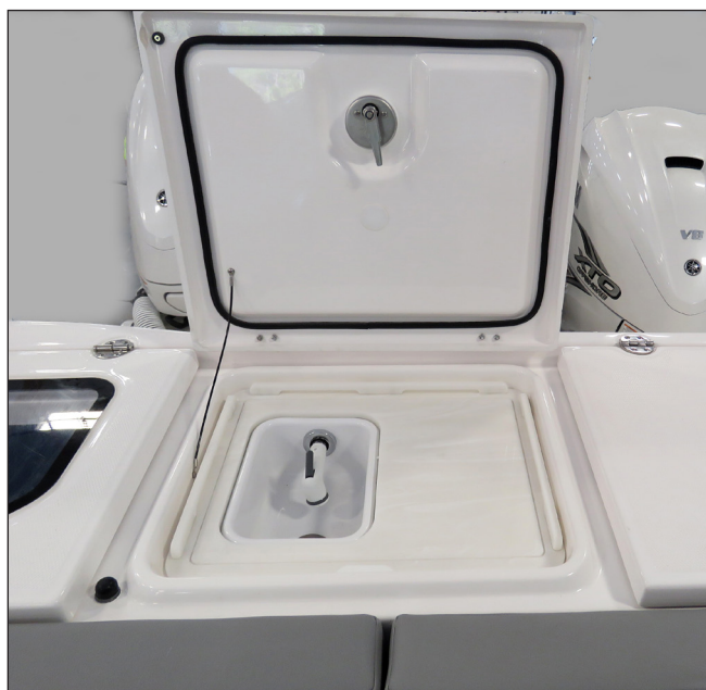
Retractable Rigging Station Retracted
