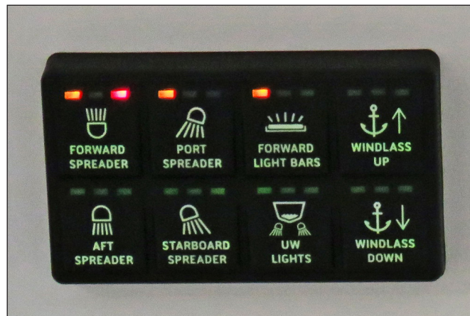
Windlass UP/DOWN Switches in Hardtop Switch Panel
