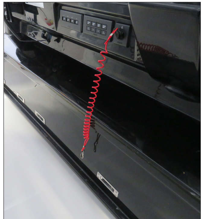
Quad Engine Stop Switch Lanyard
