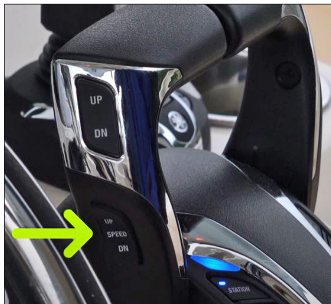
Yamaha Engine Speed Up/Down Control
