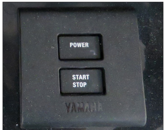
Helm Master POWER & All Engine START/STOP switches Radio Frequency ID Key Activated
