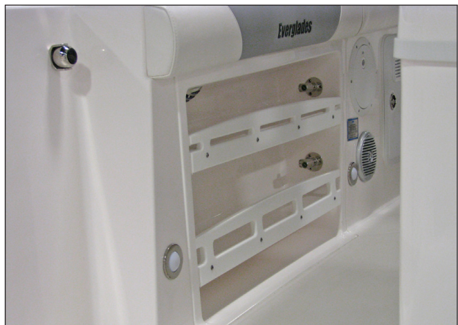
Freshwater & Raw Water Washdown Connections
