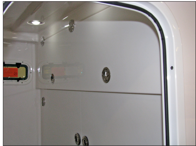
Opening Access Panel to Service Helm Components & Access Fuss Panels
