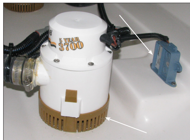
Bilge Pump Strainer and Automatic Switch
