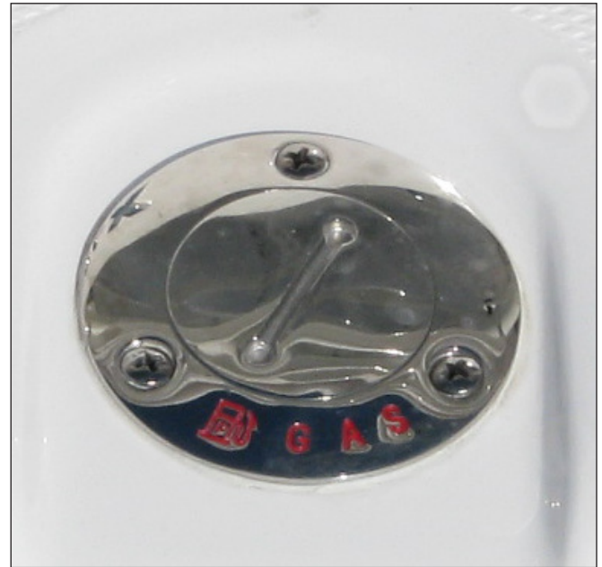
Typical Fuel Fill
