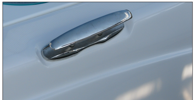
Typical Cleat in the Mooring Position
