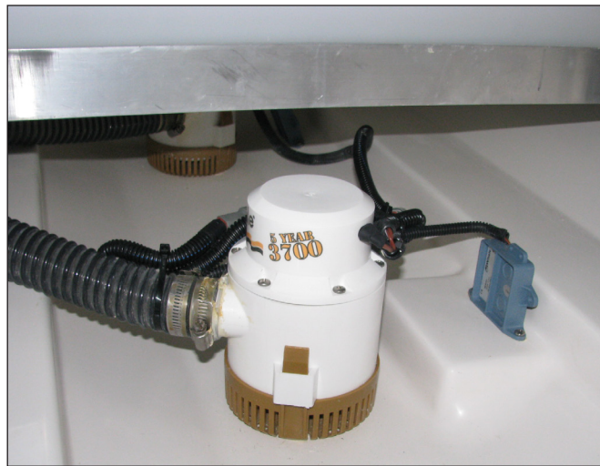
Typical Bilge Pump and Automatic Switch
