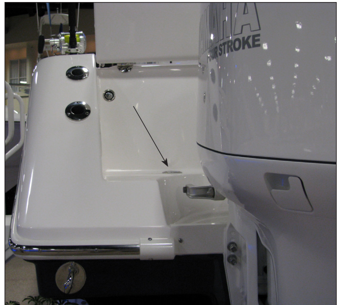
Port Splashwell Platform and Water Tank Fill
