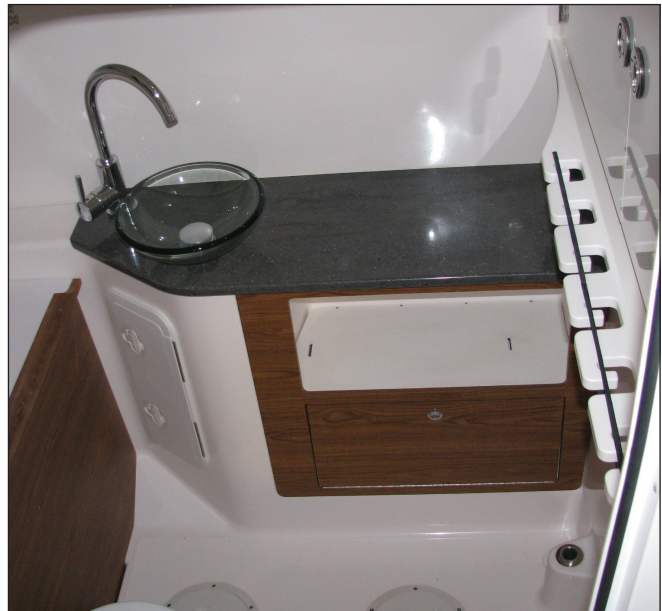
Head Compartment Vanity Sink and Faucet
