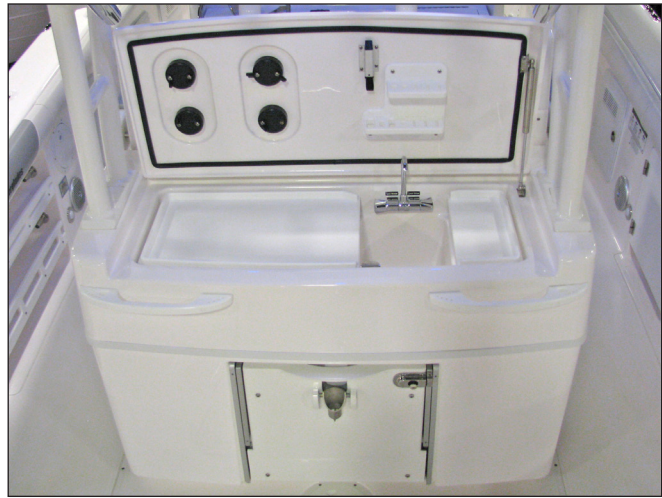
Work Station Sink with Fresh and Raw Water Sink
