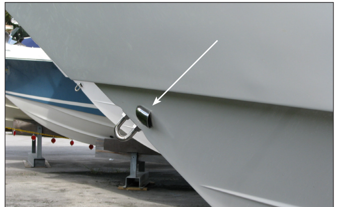
Rope Locker Drain Fitting in Hull Side
