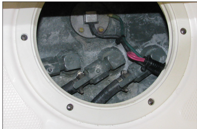
Fuel Valves and Fuel Gauge Sending Unit
