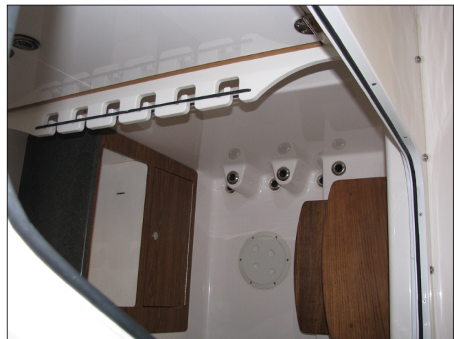
Rod Racks on Rear Bulkhead
