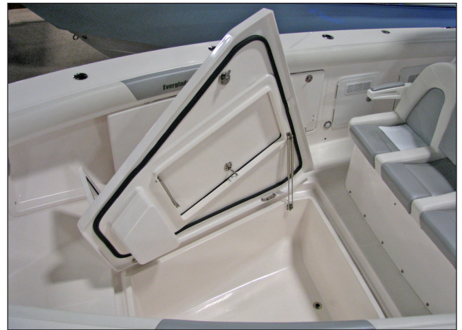
Forward Fishbox Main Hatch Open
