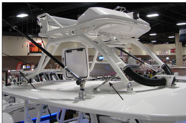
Sport Upper Station Hinge Points Showing Gas Charged Lift Assist & Dampening Cylinders
