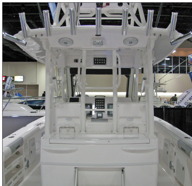
Upper Station Ladder and Work Station Showing Jump Seat/ Fighting Chair and Work Station as Steps to the Ladder Note the Grab Rails on Each Side of Ladder
