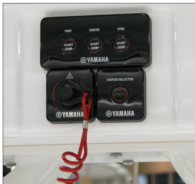
Upper Helm Engine Start/Stop Switches Engine Stop Switch & Lanyard
