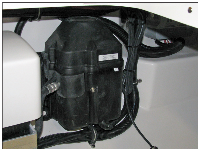
Typical Power Steering Unit in the Systems Compartment
