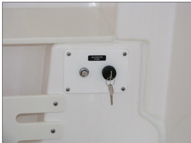
Waste System Pump Out Switch Panel
