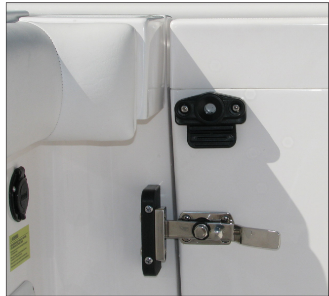
325 Center Console Dive Door Latch and Safety Pin
