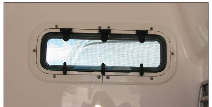
Cabin Port Window and Twist Action Locks
