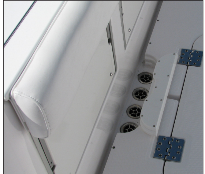
Typical Scupper Drains and Drain Rail
