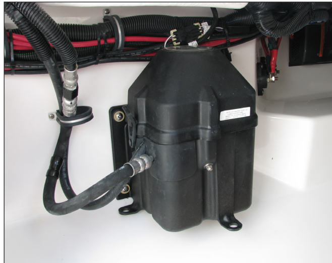
Power Steering Unit in Stern Bilge
