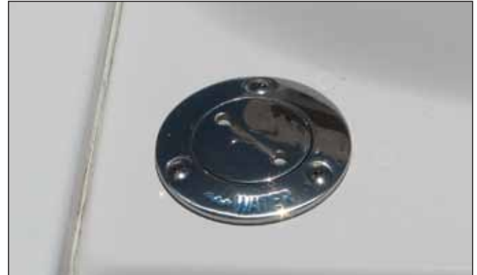
Fresh Water Fill
