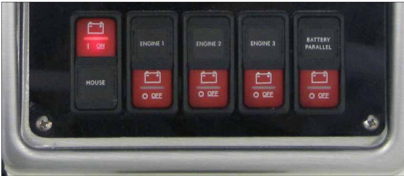
Parallel and Battery Switches in Helm Switch Panel
