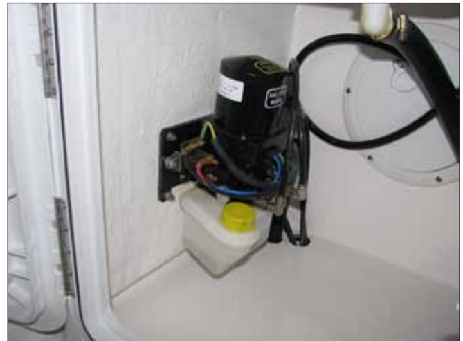
Hydraulic Pump for Windshield
