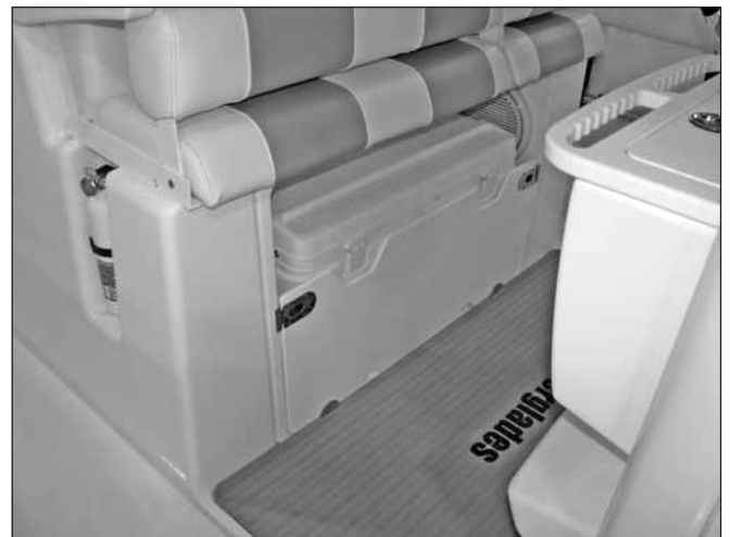
Cooler in Cooler Compartment
