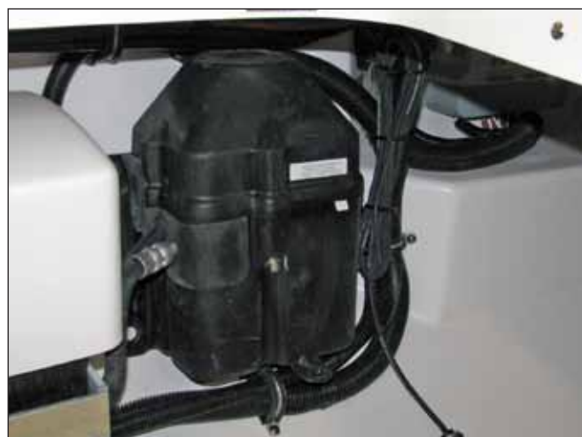
Power Steering Unit in the Systems Compartment
