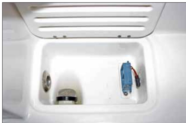
Head and Shower Sump System
