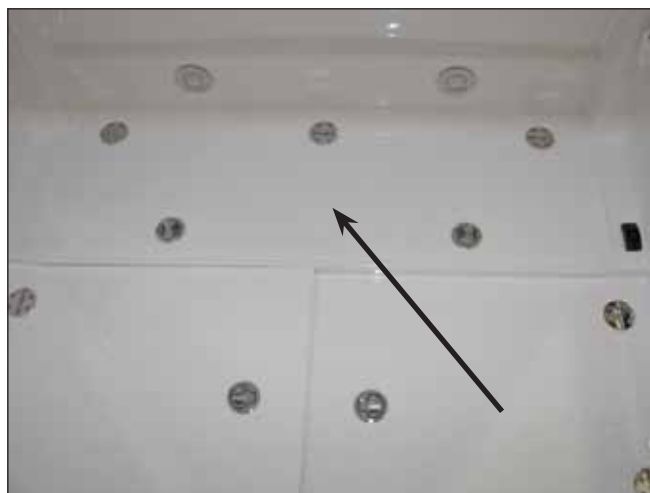
Removable Hatch to Access Back of Helm
