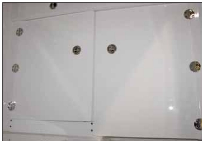
Storage Doors in Rear Head Compartment Bulkhead The Latches that Secure the Opening Helm Section are in the compartment behind these doors
