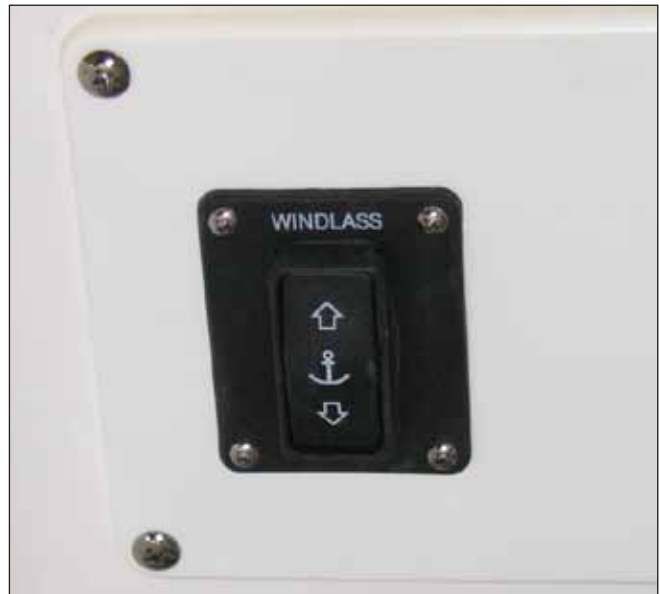
Windlass Switch in Rope Locker Near Windlass
