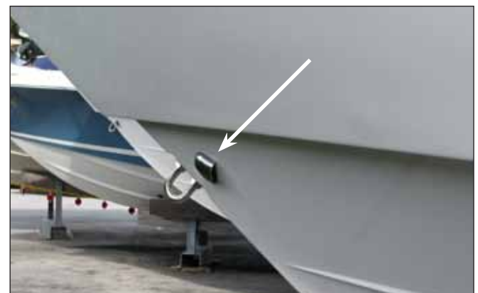
Rope Locker Drain Fitting in Hull Side
