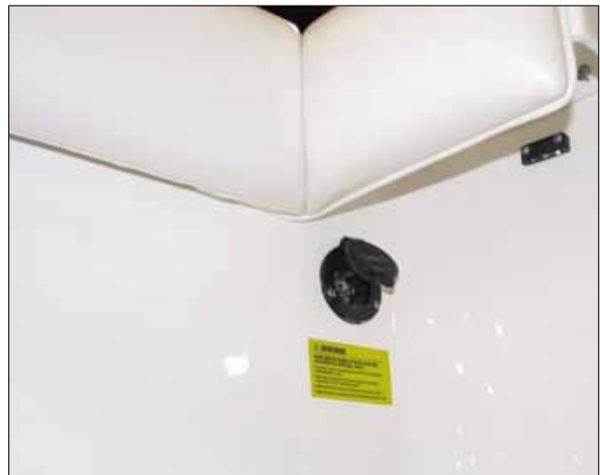
Shore Power Inlet Connection
