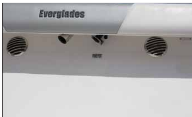
Bilge and Systems Compartment Vents
