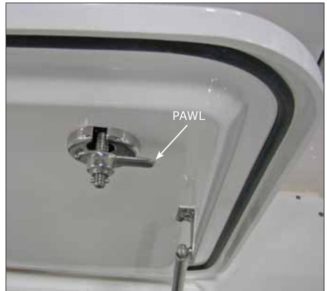
Systems Hatch Compression Latch Note Threaded Handle Shaft to Pawl
