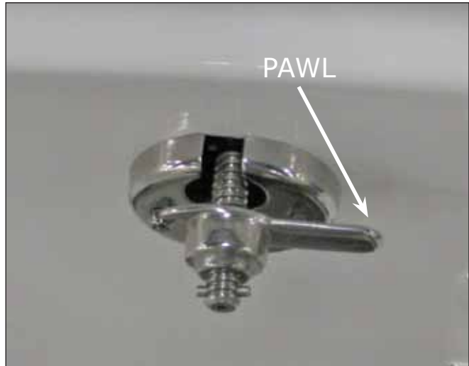
Opening Helm Section Compression Latch Note the Threaded Handle Shaft and Pawl
