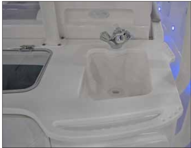
Work Station Sink with Fresh and Raw Water Shower
