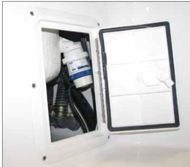
Livewell Recirculation Pump
