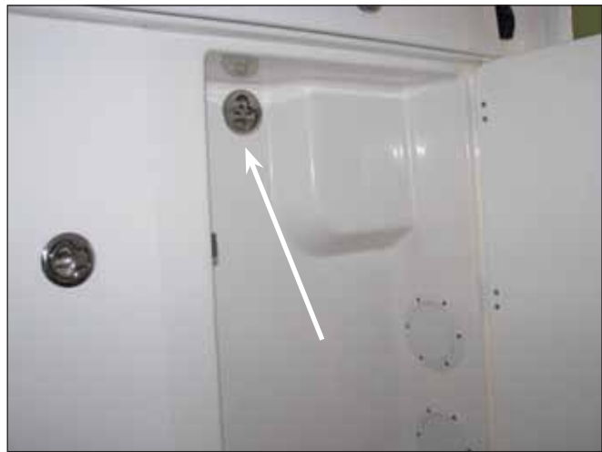
Port Opening Helm Section Latch
