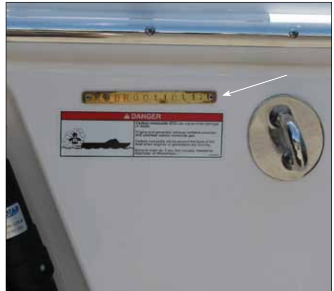
Hull ID # On Starboard Side of Transom
