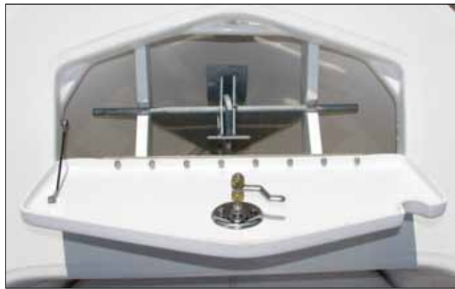
Anchor Properly Secured in Locker
