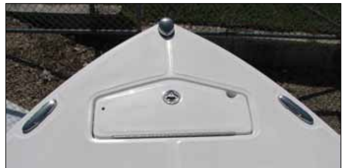
Anchor Rope Locker and Latch
