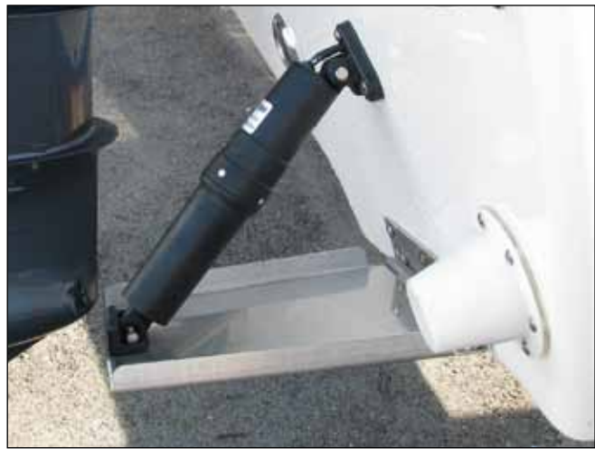
Typical Trim Tab Plane and Actuator
