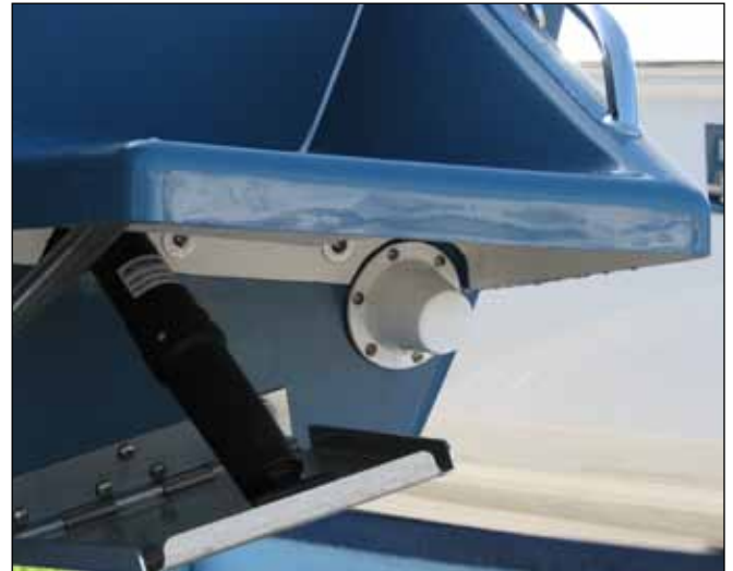
Scupper Drain Check Valve Assembly
