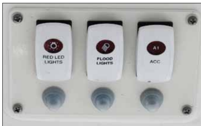
Typical Hardtop Switch Panel
