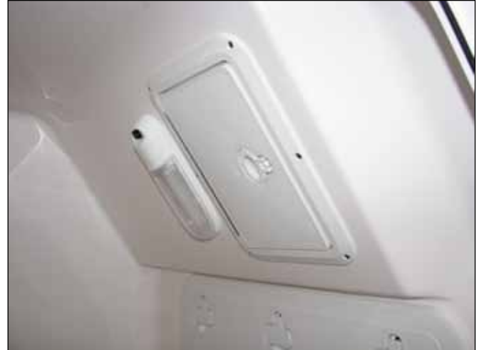
Upper Helm Access Hatch and Light Fixture
