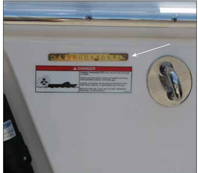
Hull ID # On Starboard Side of Transom
