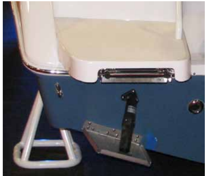
Typical Trim Tab Plane and Actuator
