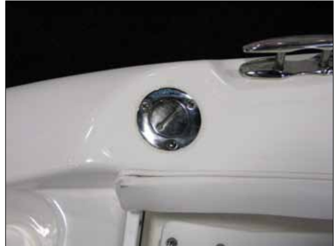
Fresh Water Fill
