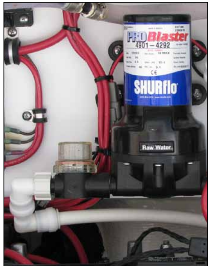
Typical Raw Water Pump and Strainer
