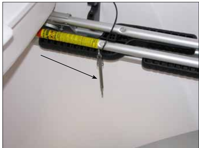
Forward Boarding Ladder Folded in Storage Bracket Storage Bracket Quick Release Pin
