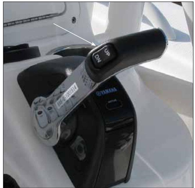
Typical Power Tilt and Power Trim Switch
