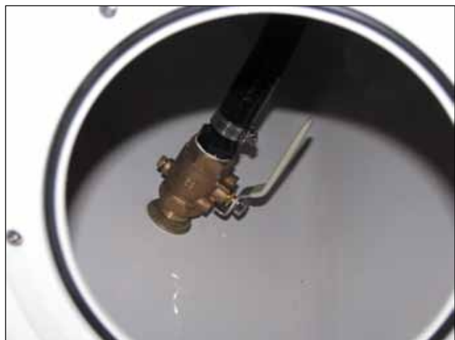
Forward fishbox Seacock Valve Behind Inspection Plate in Head Compartment
