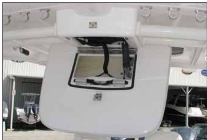
Overhead Electronics Locker Lowered for Inside Access
