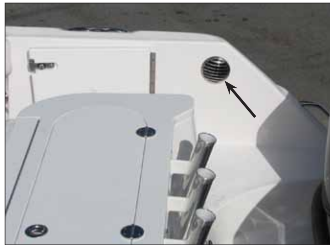
Aft Forced Air Vent
