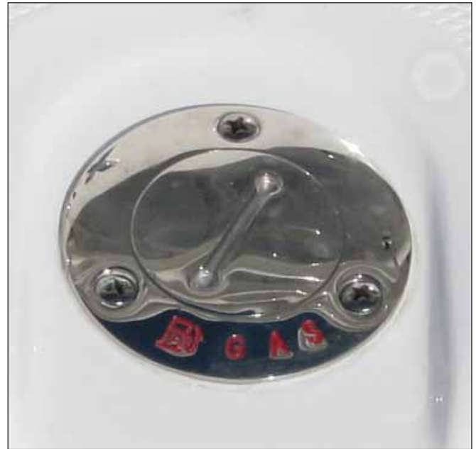
Typical Fuel Fill
