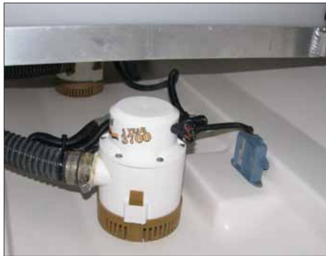
Typical Bilge Pump and Automatic Switch
