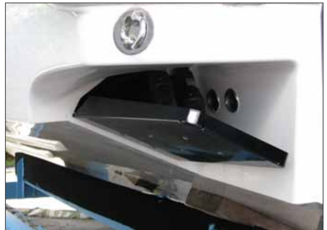
Scupper Drain Thru-hull Fittings
