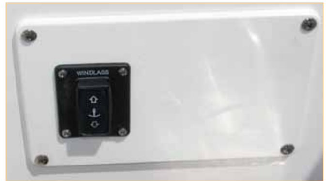
Windlass Switch in the Rear of the Rope Locker
