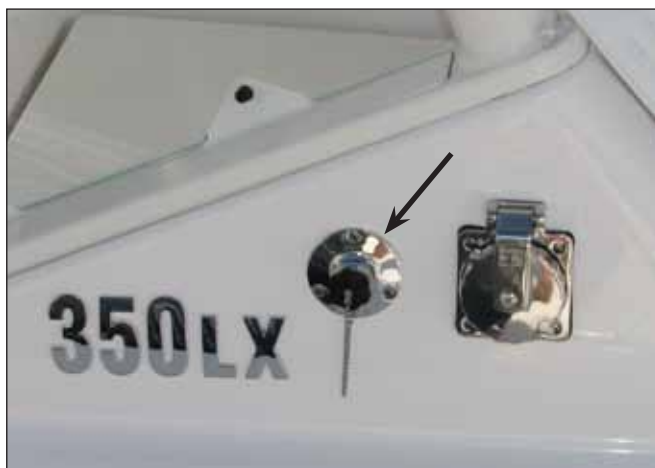
Shore Water Inlet Connection
