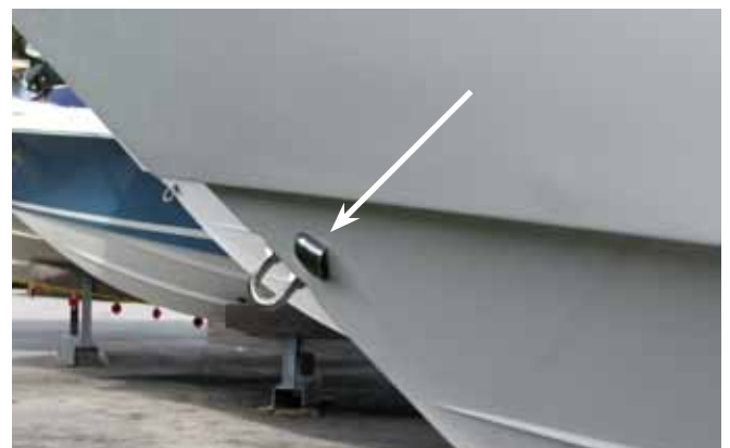
Rope Locker Drain Fitting in Hull Side
