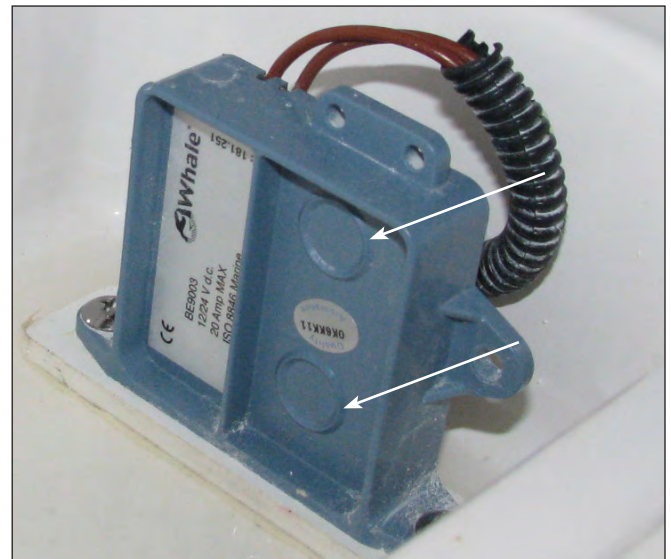
Auto Switch Test Disc Locations
