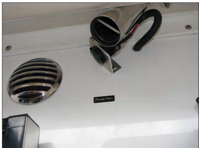
Typical Power Port Below the Gunnel inS Cockpit
