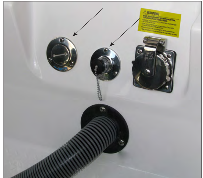
Fresh Water Fill and Shore Water Connection
