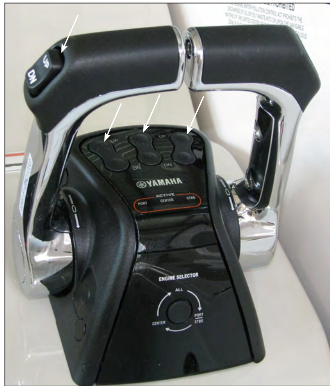
Yamaha Triple Engine Trim Switches
