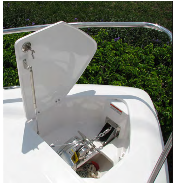
Rope Locker and Windlass
