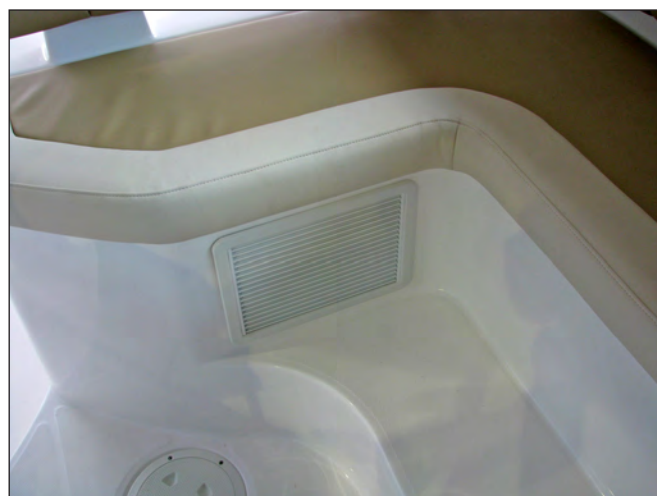
Helm Air Conditioning Air Intake
