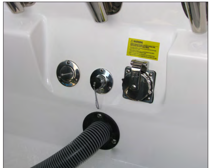
Shore Power Inlet Plug, Shore Water Connection and Fresh Water Tank Fill Fitting
