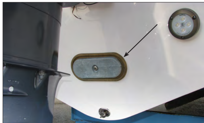
Typical Transom Anode
