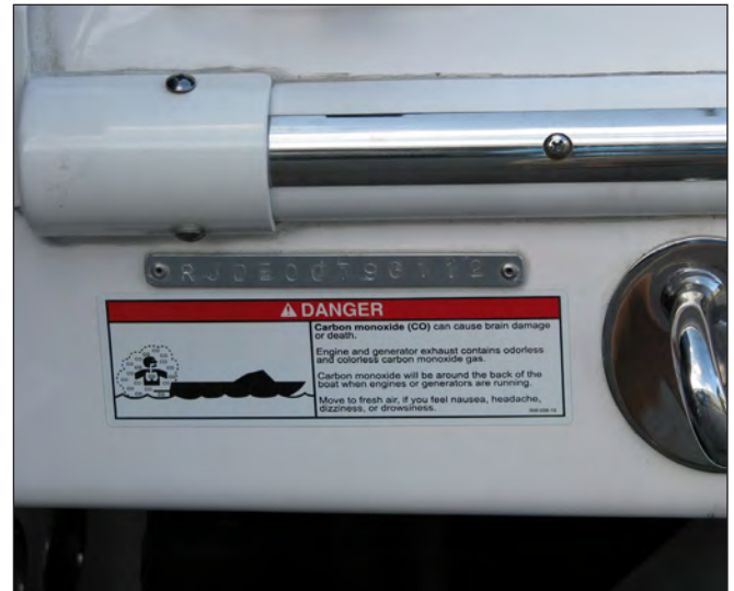
Hull ID # On Starboard Side of Transom
