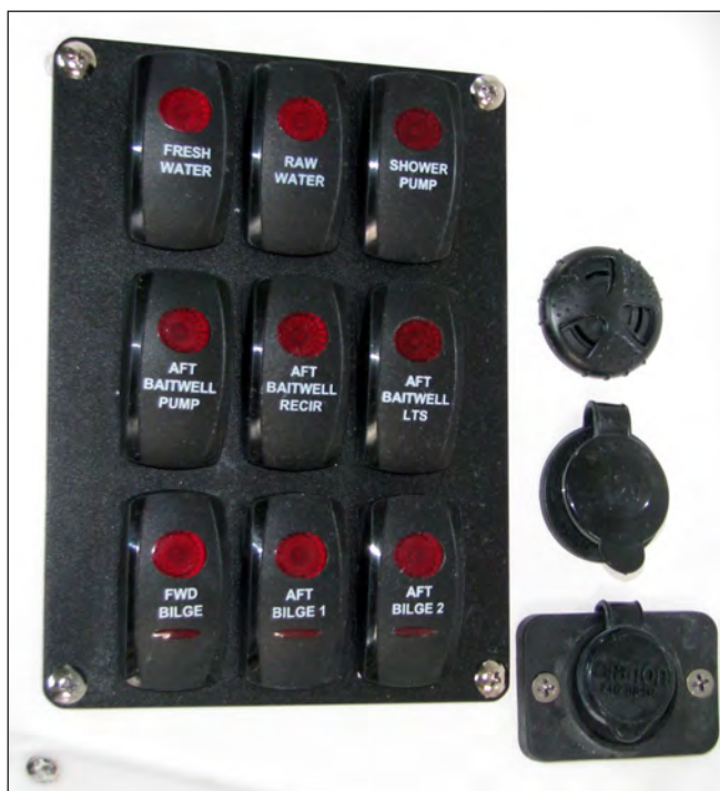
Accessory Switch Panel 2, Engine Alarm, Accessory Plug and MP3 Connection in Storage Compartment on Starboard Side Of Helm
