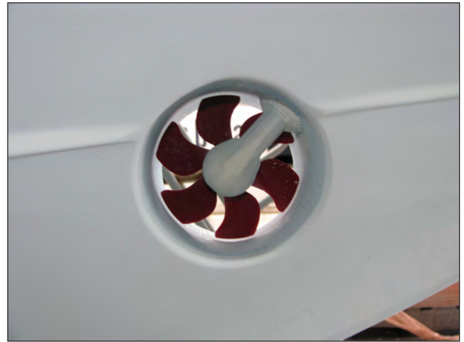
Typical Bow Thruster Drive Unit, propeller and tunnel
