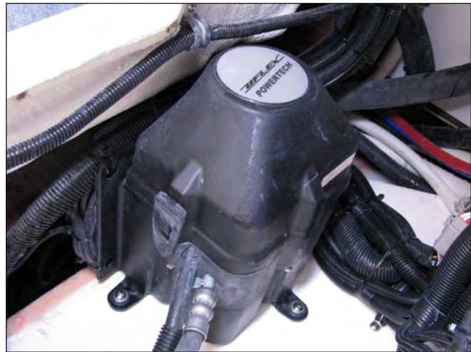
Power Steering Unit in Compartment on Starboard Side of the Helm
