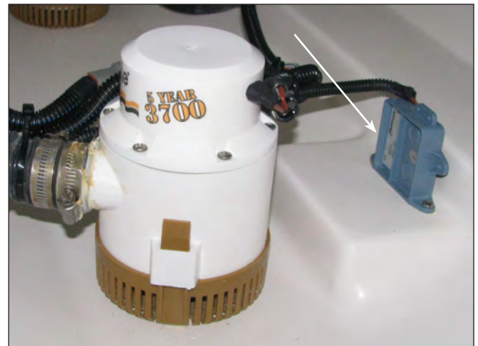
Bilge Pump Strainer and Automatic Switch
