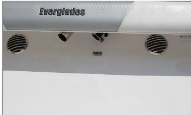
Bilge and Systems Compartment Vents
