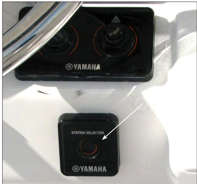
Typical Yamaha Station Transfer Button
