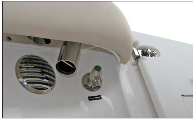
Typical Washdown Hose Connection
