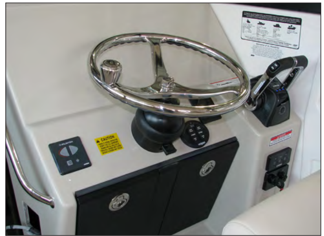
Typical Tilt Steering Wheel
