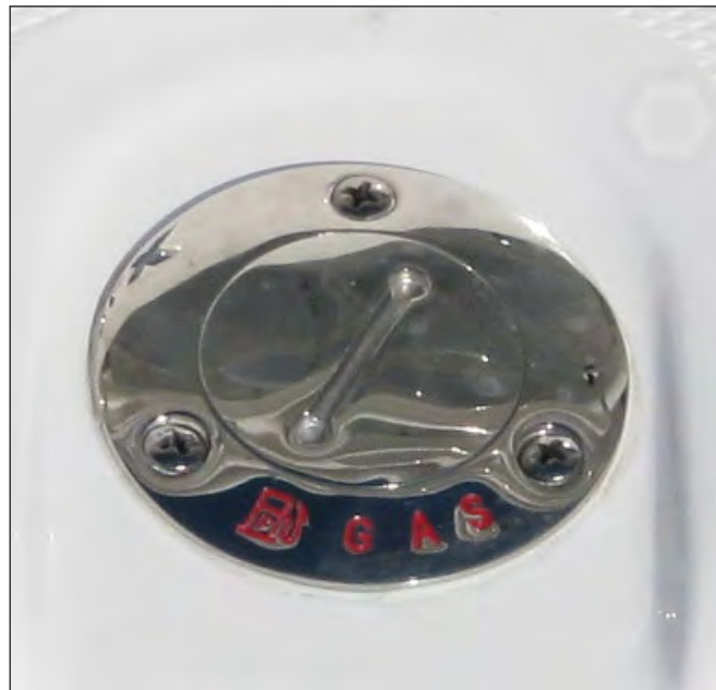
Typical Fuel Fill
