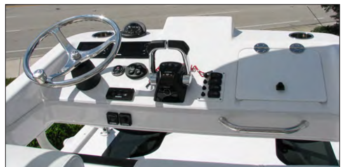
Typical Upper Control Station Helm
