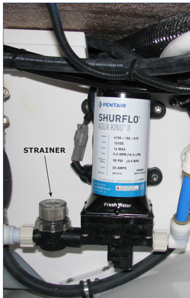
Raw Water Pressure Pump & Sea Strainer
