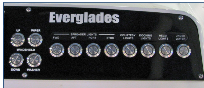
Starboard Side Helm Switches
