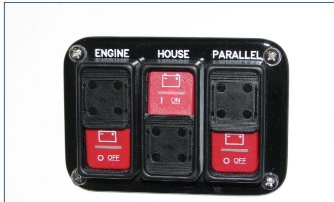
Remote Battery Switches
