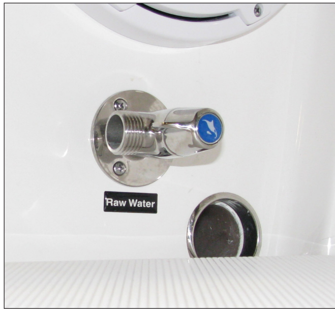
Typical Washdown Hose Connection
